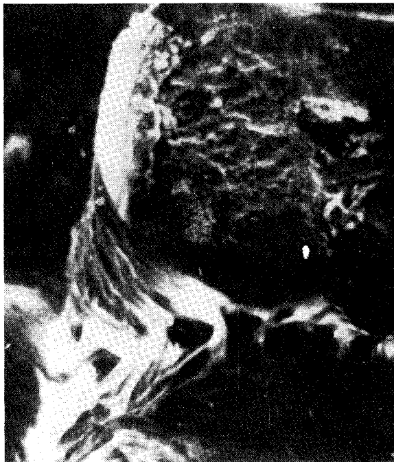
Fig. 5 Primary and secondary cracks in a fiber cross section, and matrix striations at the interface.
